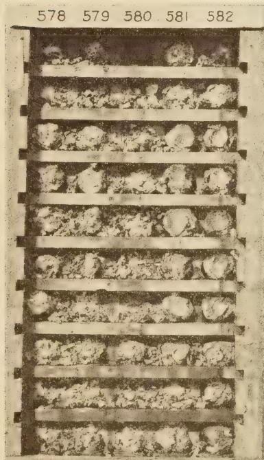
Cylinders with Truscon and BaCl 2 admixed as follows, after three years in lake: Series 578.—1 per cent Truscon Series 579.—2 per cent Truscon Series 580.—4 per cent Truscon Series 581.—6 per cent BaCl 2 Series 582.—12 per cent BaCl 2
